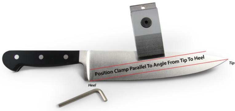
**PRO TIP :** For proper clamp alignment place a piece of masking tape from tip to heel in such a way that the longer edge makes a straight line from tip to heel of the edge!
