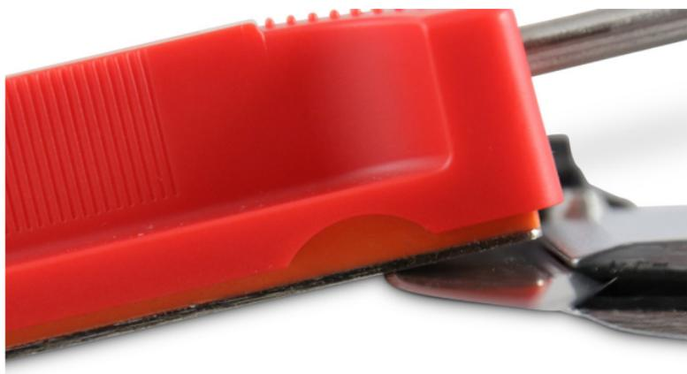
Before sharpening your knife, adjust the guide rod locking collar so that the diamond hone block sits on the knife edge when fully extended (as pictured) and stone stays in contact during a full pass across the blade.
